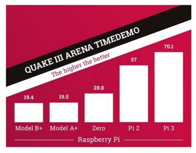
The classic twitch shooter from industry pioneer id Software, Quake III Arena is heavily tied to the CPU performance of the Pi. The standard 'timedemo' was run at 1280×1024, high geometric, maximum texture detail, 32-bit texture quality, and trilinear filtering to obtain these results.
