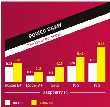
You can't get extra performance without a few sacrifices. The Pi 3 draws the most power of the test group, but its extra performance means it spends more time at idle. Those looking for maximum battery life should look at the Model A+ or the Pi Zero as an alternative.
