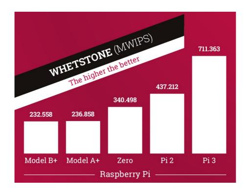
Developed by B.A. Wichman in the 1970s as a means of measuring a computer's speed, the Whetstone benchmark concentrates on floating-point performance. Despite its age, the benchmark offers a good insight into the peak floating-point performance of a processor.
