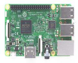
The headlining feature of the Pi 3 is the built-in WiFi and Bluetooth, but it doesn't stop there. Here's the complete spec for the Pi 3:
