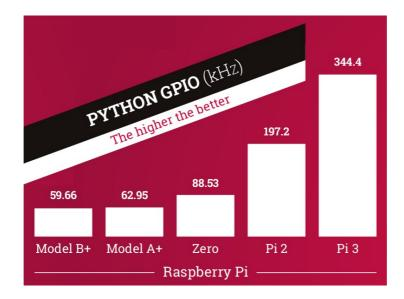
The Raspberry Pi's GPIO pins are most commonly used with Python, but this leads to a CPU bottleneck. In this test, a simple RPi.GPIO program toggles a pin as rapidly as possible while a frequency counter measures how quickly it actually switches.
