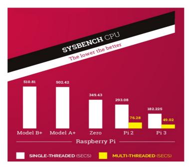
Offering support for multi-threaded operation – taking advantage of the four processing cores on the Pi 2 and Pi 3 – SysBench reveals just how far we've come since the original Raspberry Pi design. While single-threaded performance has improved greatly, the biggest gains go to multi-threaded programs.
